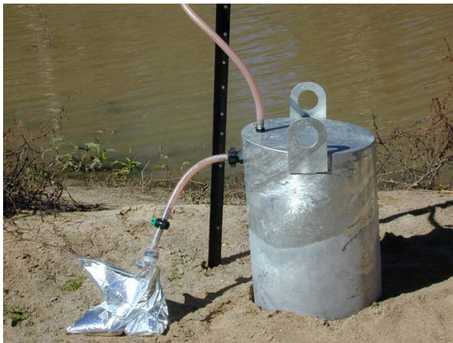
Figure 4: Basic components of the seepage meter including seepage chamber and collection bag
